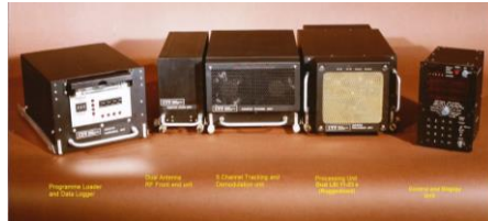
The STL designed Navstar receiver as supplied. Trialled in Tornado, Type 42 and Submarines
